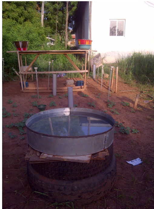
Figura 2. Plate 1. Growing melon plant with installed evaporimeter .
