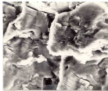
d. Fracture surface detail. The direction of crack growth at the level of material grains is evident (x3000)
