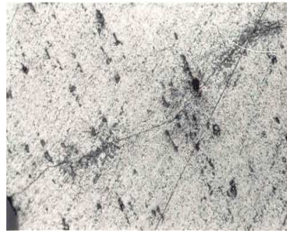
b. Metallographic micrograph showing different manganese compounds developed within the immediate area of the fatigue crack (x400)
