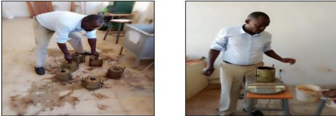
Figure 11: CBR testing in the laboratory
