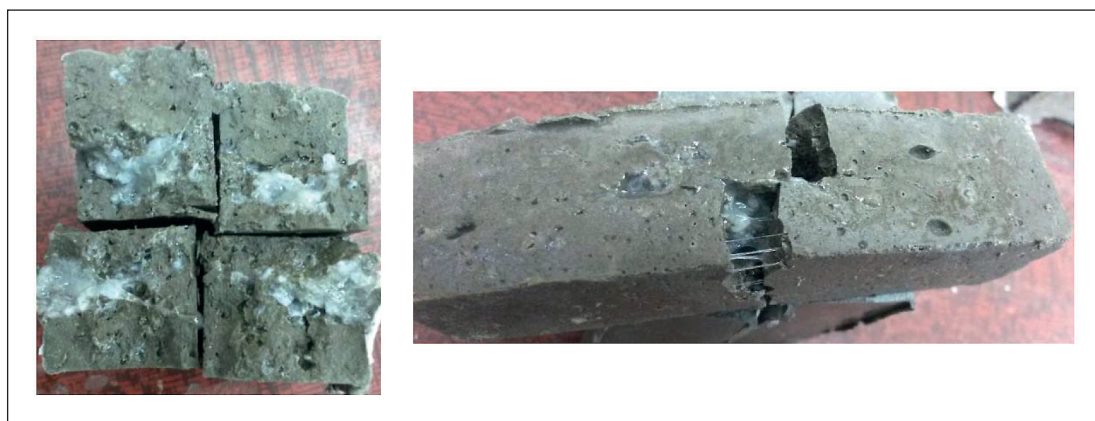
Fig. 2. Samples of cement stone containing PAA (1%)
