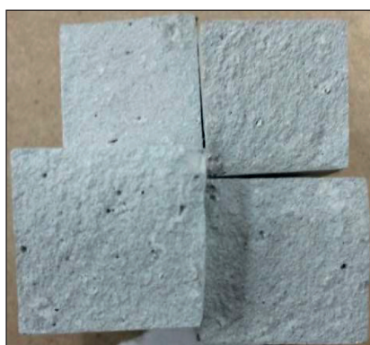
Fig. 6. Samples of cement stone containing SP (1%)
