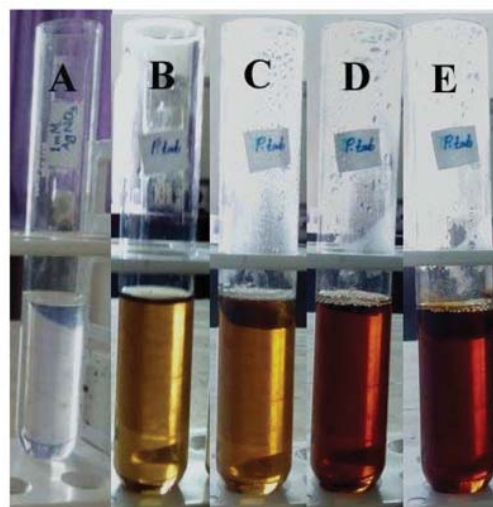
Fig. 2. A — \text{AgNO}_3 solution; B — mixed \text{AgNO}_3 and extract; C — colour transformation after 30 min; D — colour transformation after 1 hour; E — colour transformation after 2 hours
