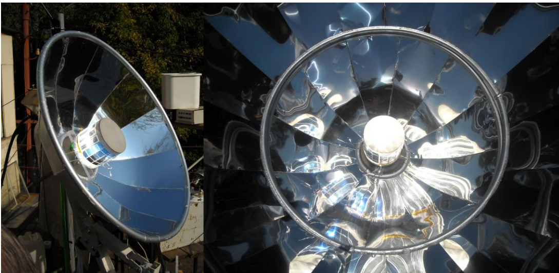
Fig. 10. Solar photovoltaic thermal module with a concentrator of paraboloid type
