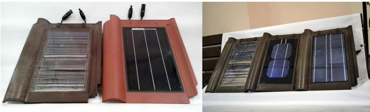
Fig. 3. Roofing solar panels of two types with extended service life
