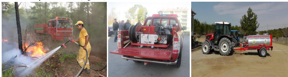
Figure 7: Sprinkler Truck, First Responder Vehicle and Fire Extinguisher Tank
