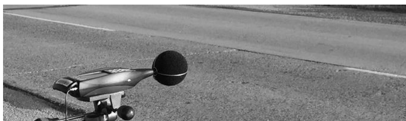
Fig. 3. View of the Bruel & Kjaer 2250 sound analyser in one of the places where measurements were taken
