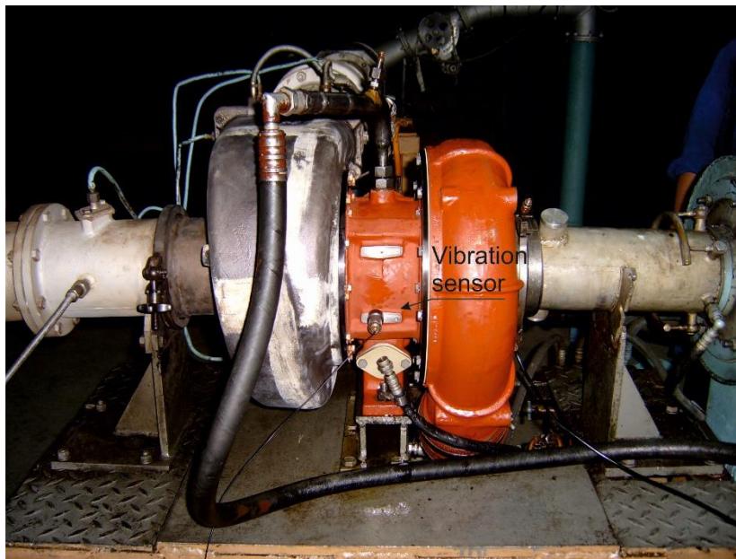
Fig. 1. Stand test for C0-45 turbochargers and the vibration sensor
