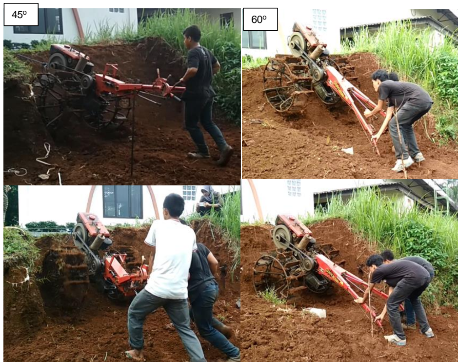
Fig. 12 - Differences in the handle position of adjustable handlebar and fixed handlebar
