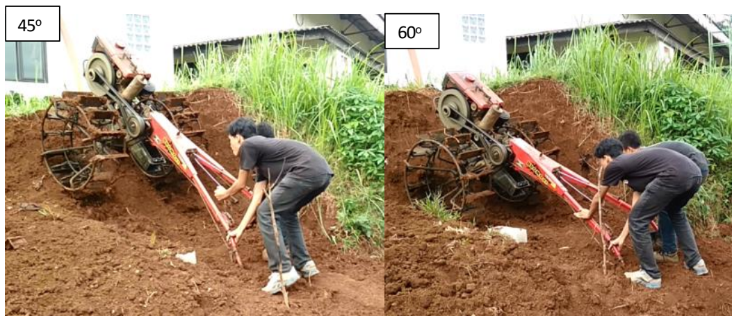
Fig. 11 - Handle position using handlebar without hinge while climbing 45° and 60° slope
