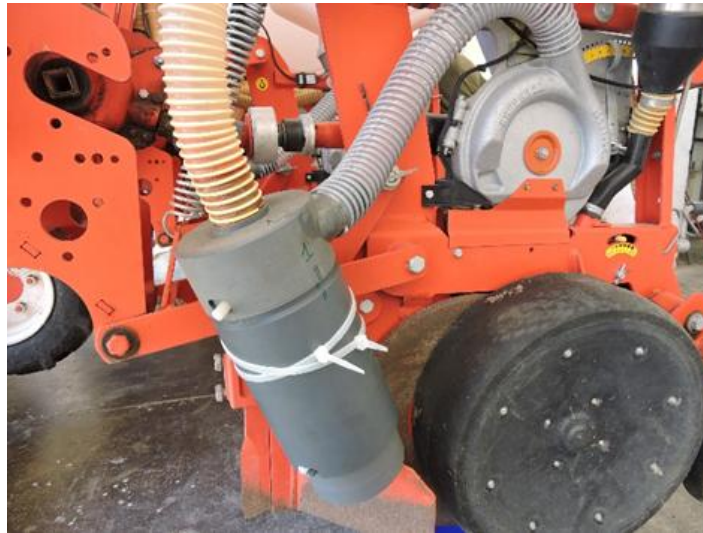
Fig. 4 - The small cyclone mounted before the seed heads proposed by ILVO
