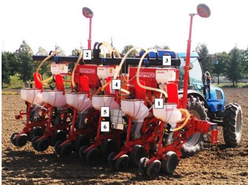
Fig. 5 - Modified drill with the recycling-filtering device proposed by CREA.
