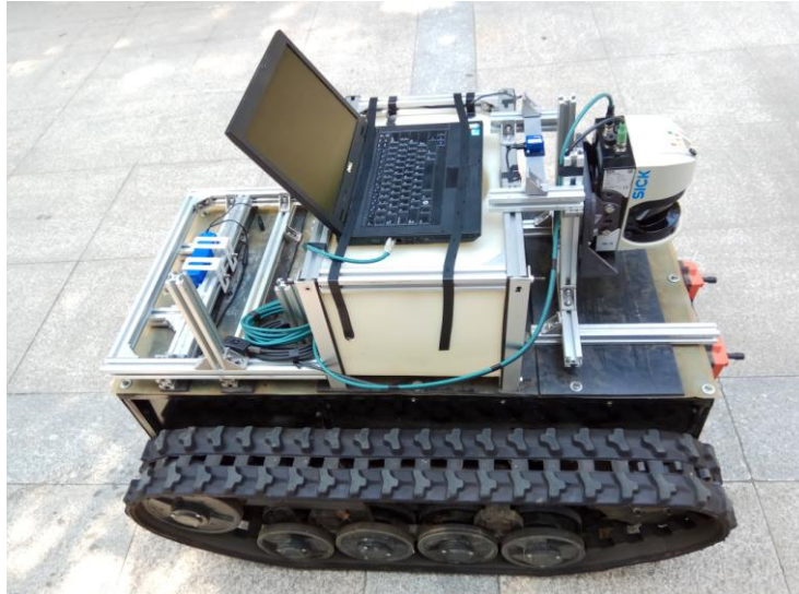
Fig.4 - The structure of forest precise positioning mobile platform Laser scanner; Attitude and heading reference system; Portable computer
