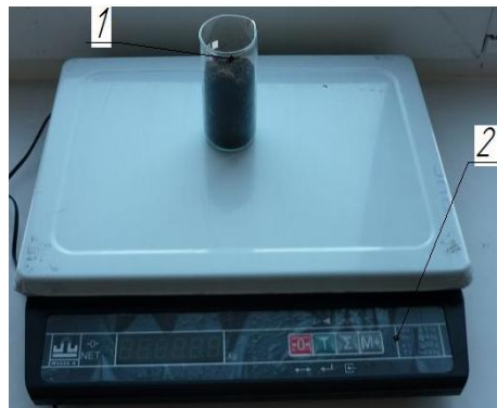
Fig. 6 – Electronic desktop scales MK-15.2-A21 1 – a glass bulb; 2 – electronic table scales
