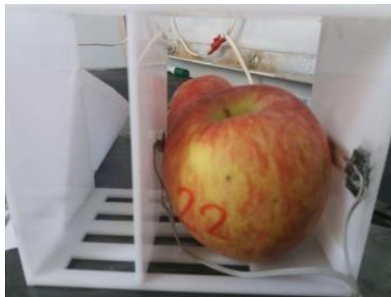
Fig.1- Non-destructive set-up to evaluate bruises
