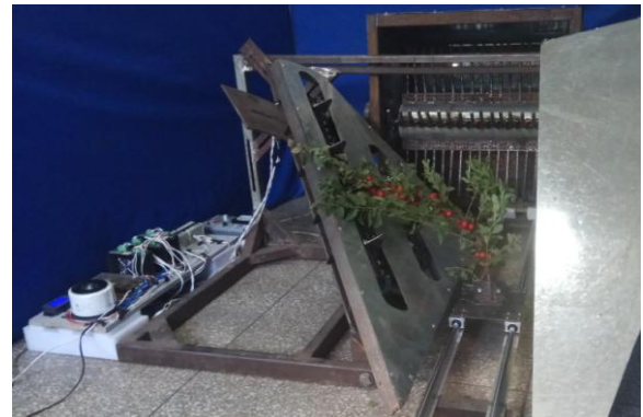
Fig. 2 - The branches lifter test bench of Cerasus humilis
