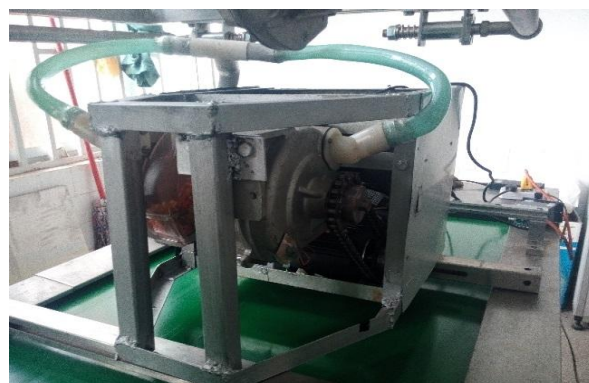
Fig. 7 - Test bench of the seed metering device performance
