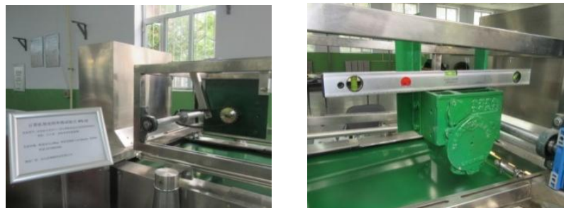
(a) volume-variable hole precision seeder; (b) bristle brush wheel seeder.
