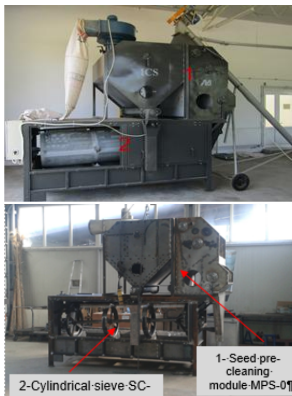
Fig. 2 – ICS seed conditioning installation
