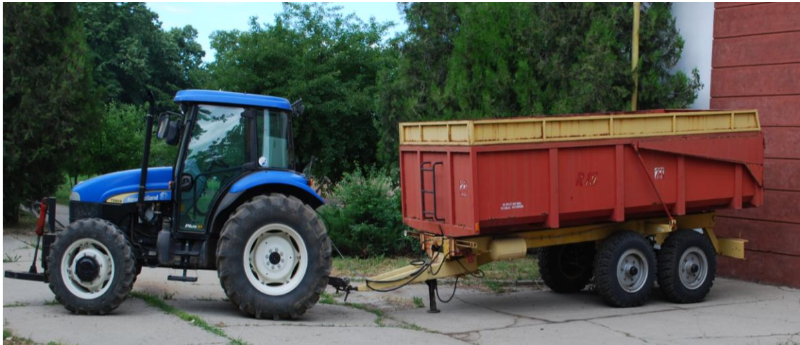
Fig. 3 – Articulated vehicle: New Holland TD80D agricultural tractor and agricultural semi-trailer
