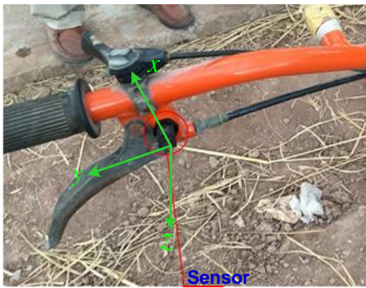
Fig. 1 - Sensor in the mini tiller and connection relation for different components
