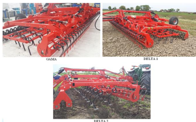
Fig. 3 - The prototype vibro-combinator SANDOKAN 2 equipped with the three types of active parts (GAMA, DELTA1, DELTA2)
