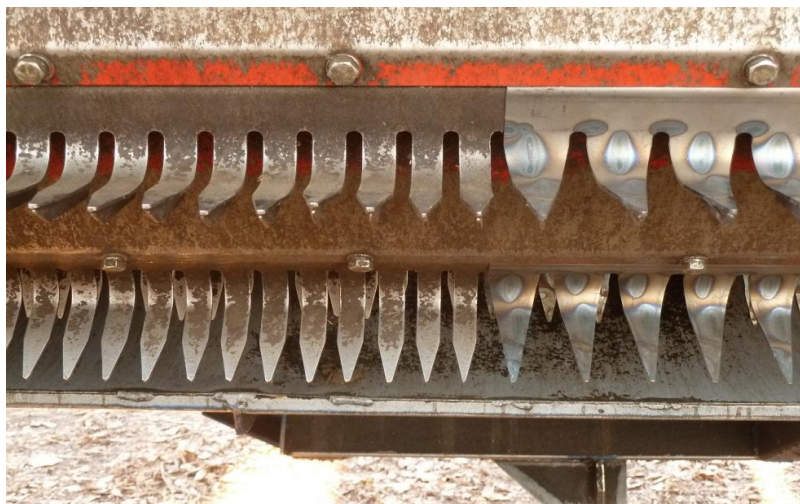
Fig. 4 - Stripping fingers of the "OZON" header (Russia): left – conventional; right – modernized with large spacing between tines
