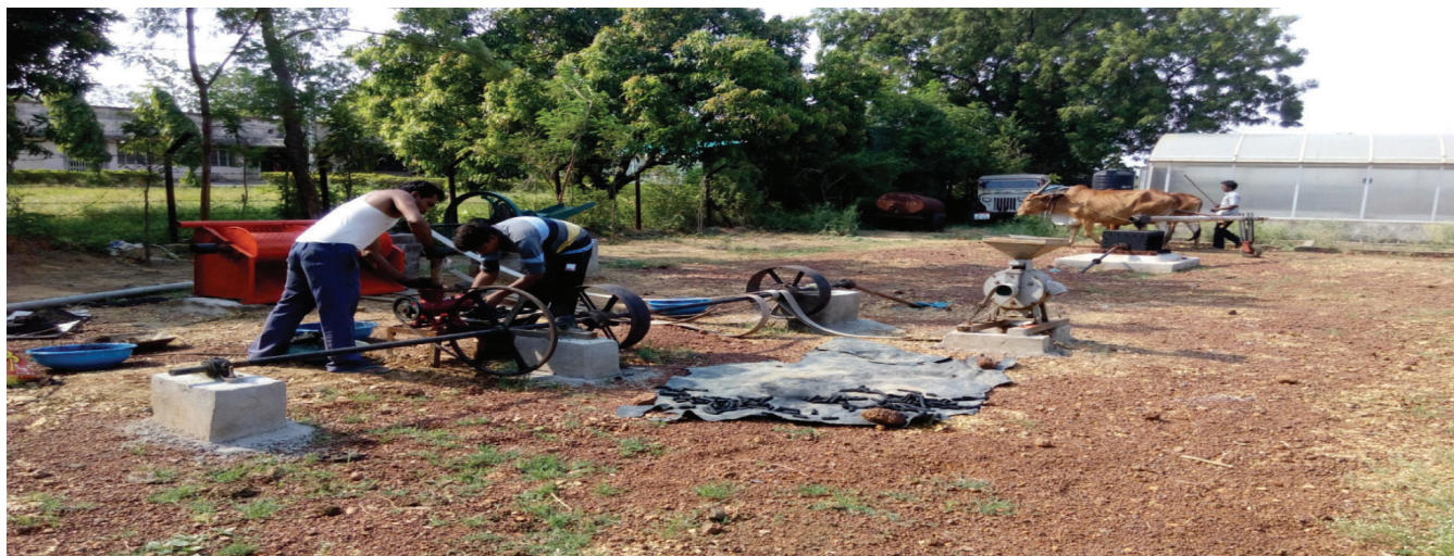
Fig. 1: Setup of rotary transmission system for measurement of draft, speed and power output during briquette production
