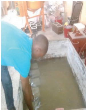
Fig. 4 – Curing of concrete cubes
