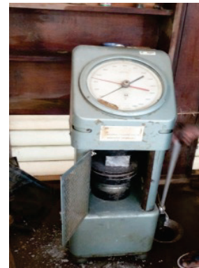
Fig. 6 – Compressive strength test
