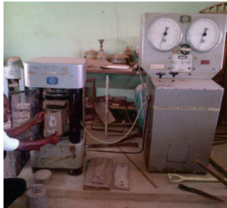
Fig 9: Compressive strength of sandcrete blocks
