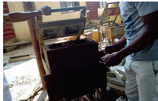
Fig 7: Block sample using hand ramming method
