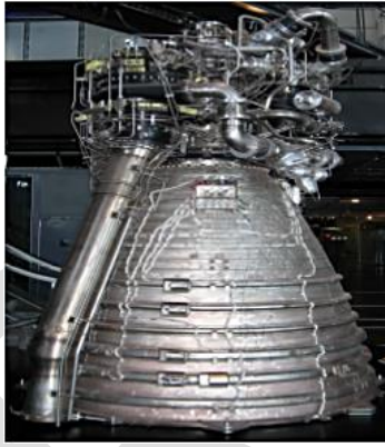
(Fig.1 Cryogenic engine /Source: Cryogenic Technology Development for Exploration Missions by David J. Chato)
