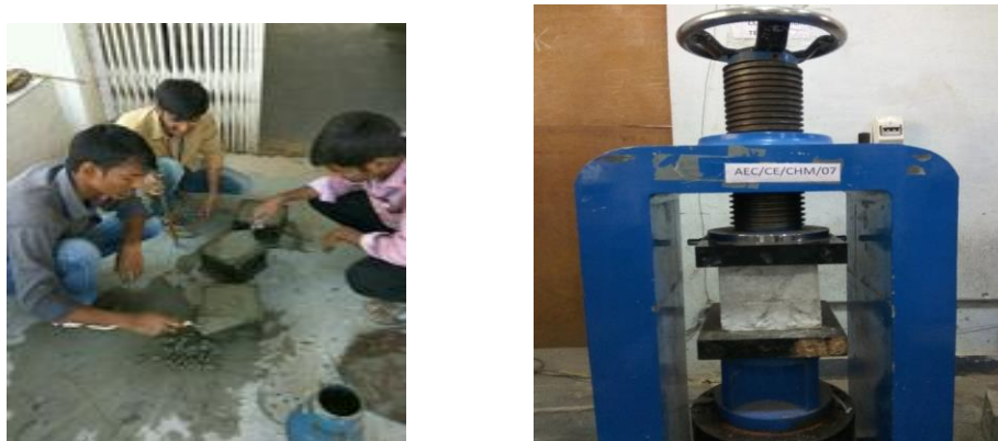
Fig 3: Casting and compressive strength testing of cube
