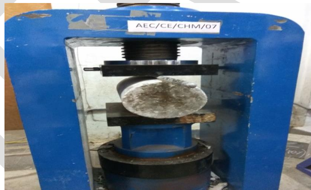
Fig 4: split tensile strength testing of cylinder
