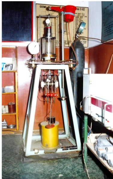
Figure 1 - Device for testing of soils under conditions of triaxial compression design Anbergen M. I.
