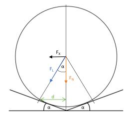
**Fig 6.** Ball-on-plate friction measurement function principle (adopted from [18]).
