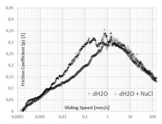
**Fig. 9.** Compiled result for different lubricants interacting with Plateau samples with a 10 N normal force.
