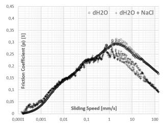
**Fig. 11.** Compiled result for different lubricants interacting with Condyle samples with a 10 N normal force.
