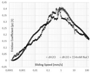
**Fig. 8.** Compiled result for different lubricants interacting with Plateau samples with a 5 N normal force.
