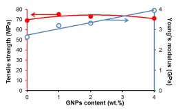
**Fig. 3.** Tensile strength and Young's modulus of PA6 filled with various contents of GNPs.
