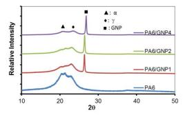
**Fig. 2.** XRD patterns of unfilled PA6 and PA6/GNP composites.
