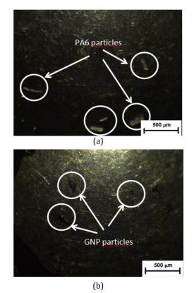
**Fig. 10.** OM images of the steel balls sliding against the (a) unfilled PA and (b) composite with 4 wt.% of GNP.
