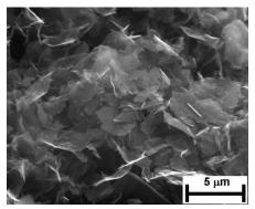
**Fig. 1.** The SEM image of GNPs.
