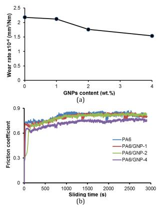
**Fig. 7.** (a) Wear rate and (b) friction coefficient of PA6 filled with various contents of GNPs.
