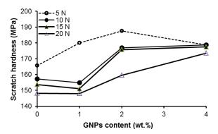
**Fig. 5.** Scratch hardness of PA6 filled with various contents of GNPs.
