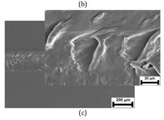
**Fig. 6.** Low and high magnification SEM micrographs of scratch scars generated on the (a) unfilled PA6, (b)
