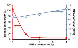
**Fig. 4.** Elongation at break and microhardness of PA6 filled with various contents of GNPs.
