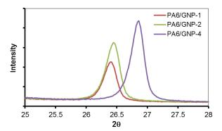
**Fig. 8.** Comparison of GNPs' XRD Bragg peak at  $2\theta$ ~26.5 deg, confirming morphological differences of the composites containing 1, 2 and 4 wt.% of GNP.
