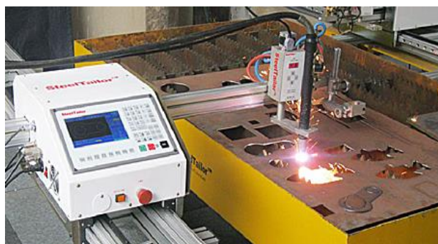
Fig. 1. CNC Steel Taylor plasma jet cutting machine.
