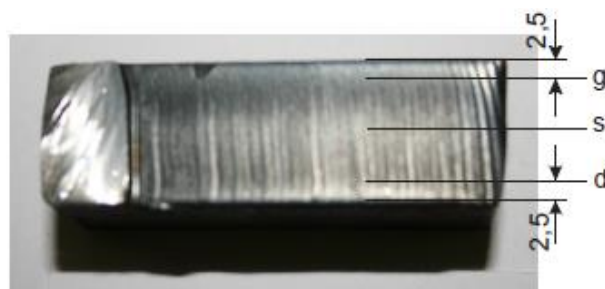
Fig. 4. Surface roughness measurement places.
