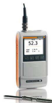
Fig. 3. Feritscope FMP 30 (Finland) with probe. Magnetic induction method is the basis of such measurement [15,16,26]. Proportions of delta
