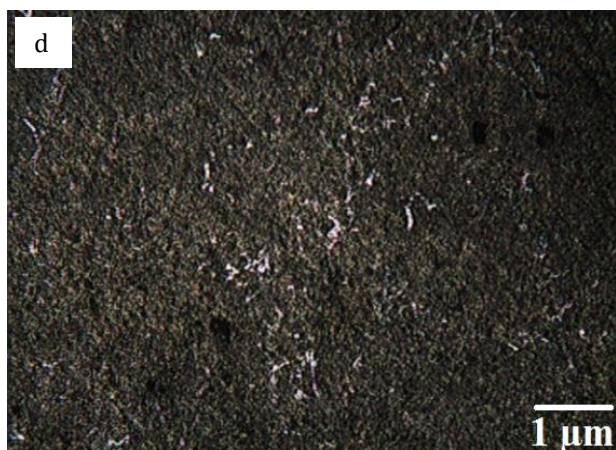
Fig. 4. Microstructure of the FGM at various distances from outer periphery a) 1 mm, b) 6 mm c) 12 mm and d) 18 mm.
