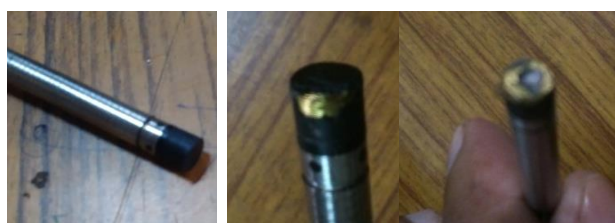
(a) Good Sensor (b) Failed Sensor
