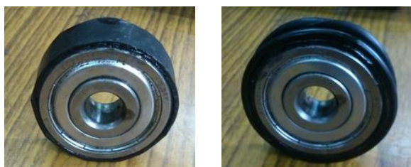
(a) Bearing with elastomer (b) Bearing with O-ring
