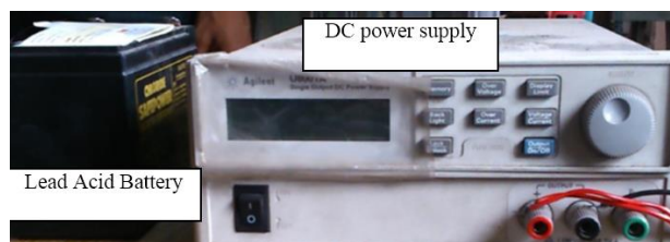
(a) Lead acid battery and DC power supply
