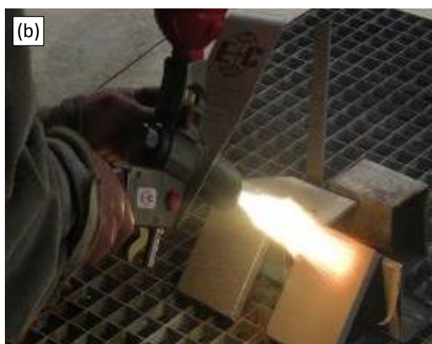
Fig. 1. Experimental setup for: (a) PTA deposition and (b) FS deposition.
