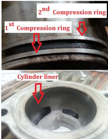
Fig. 1. Piston rings and cylinder of motor engine.
