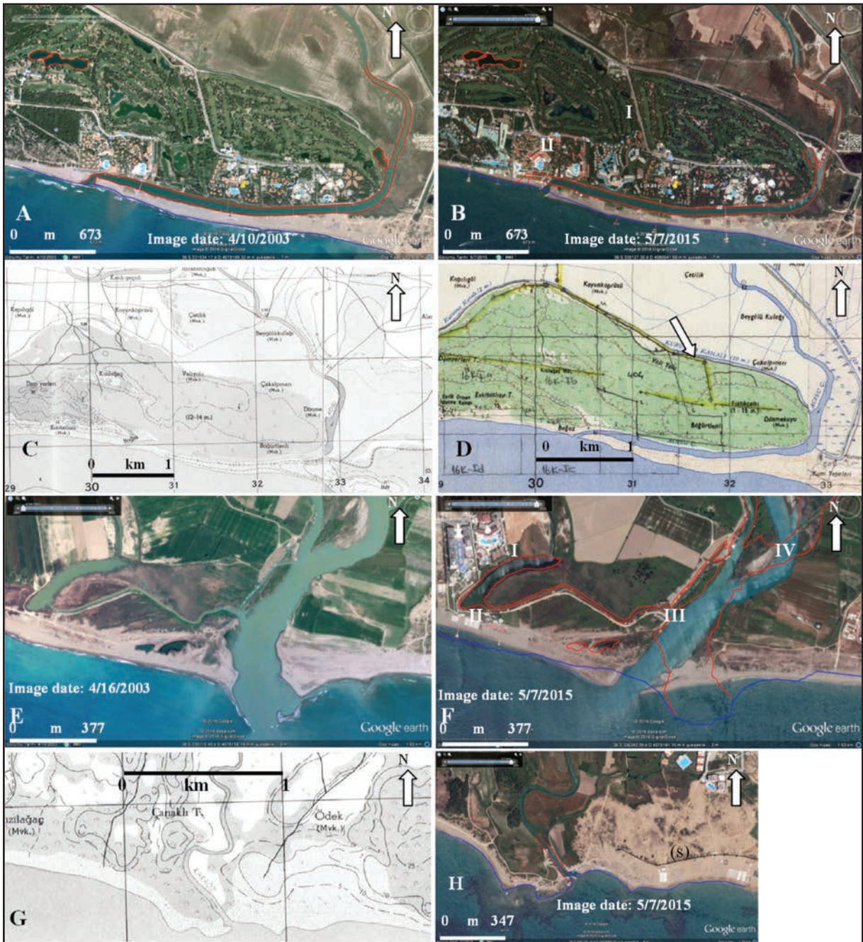
Figure 4- Google Earth satellite views of 2003 and 2015, past and recent topographic maps for the Ağılısu (A-D), Köprüiçay exit-Karaöz Stream exit (E-F), Google Earth view of south of Kısalar location, black line may be thought as wave effect boundary in last decade, numbers show changes in time.
