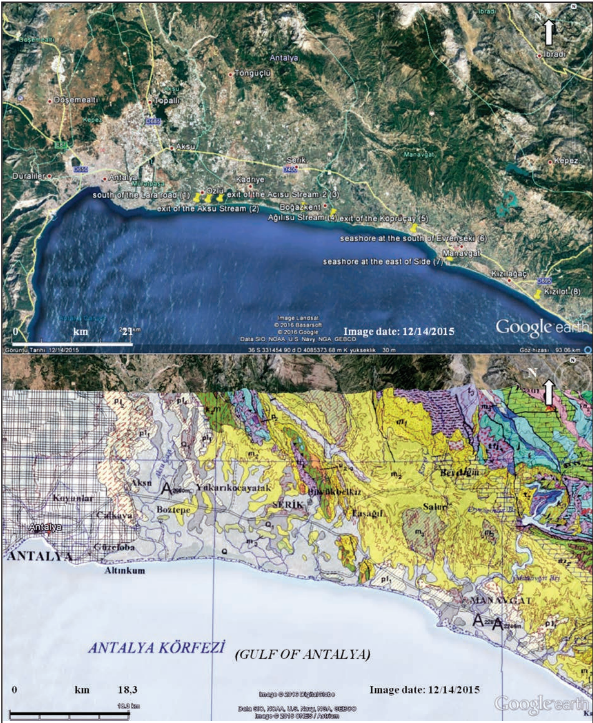
Figure 1- A map showing the studied locations (www.googleEarth) and geological map of the area on the satellite view (travertine outcrops having narrow coastal side around the Antalya, particularly low plains at the eastern parts of the Antalya, Miocene to Pliocene aged basement geological units are seen in the region, k2m. Cretaceous ophiolitic melange, e2-3. Eocene neritic limestone, m3. Miocene aged, ancient marine siliciclastic sediments, pl1. early Pliocene aged terrestrial, occasionally marine clastic sediments, Q. Quaternary alluvium, travertine-terrestrial, please see MTA geological map 1/500.000 in scale for other detail explanations of the map.
