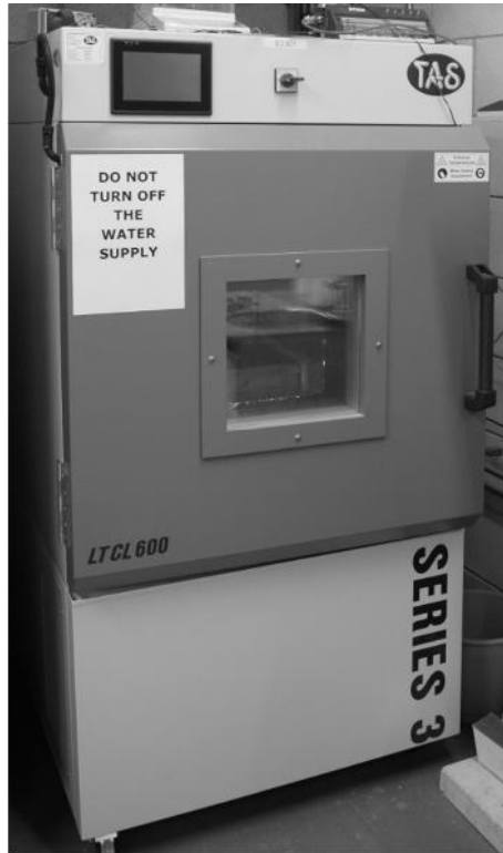
Fig.3. Climatic chamber Source: Author's
