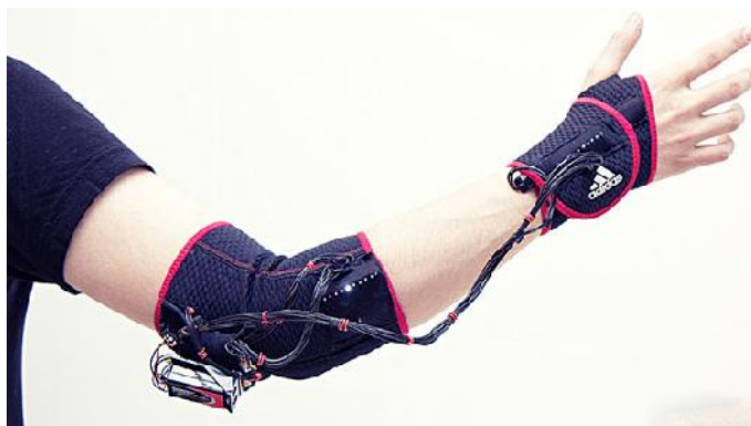
Fig. 10 The 'Ghost' system for stimulation of blind people's hand movements Source: [27]
