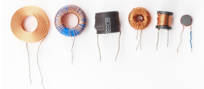
Fig. 2. Different coil types used in Buck-Converter research, from left: air coil, DTMSS coil, bigger bobbin coil, DTP coil, smaller bobbin coil and SMD coil
