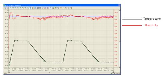
Fig. 5. The temperature-humidity curve controlled with expert control algorithm
