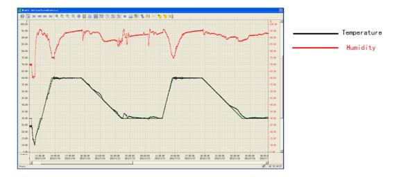
Fig. 4. The temperature-humidity curve controlled with conventional algorithms
