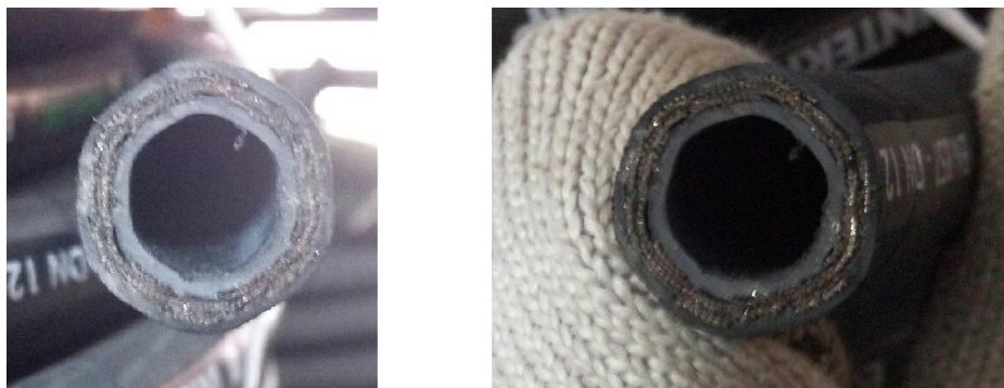
Fig. 9. The edge face cuts of the high-pressure hose after fixed cutting method
