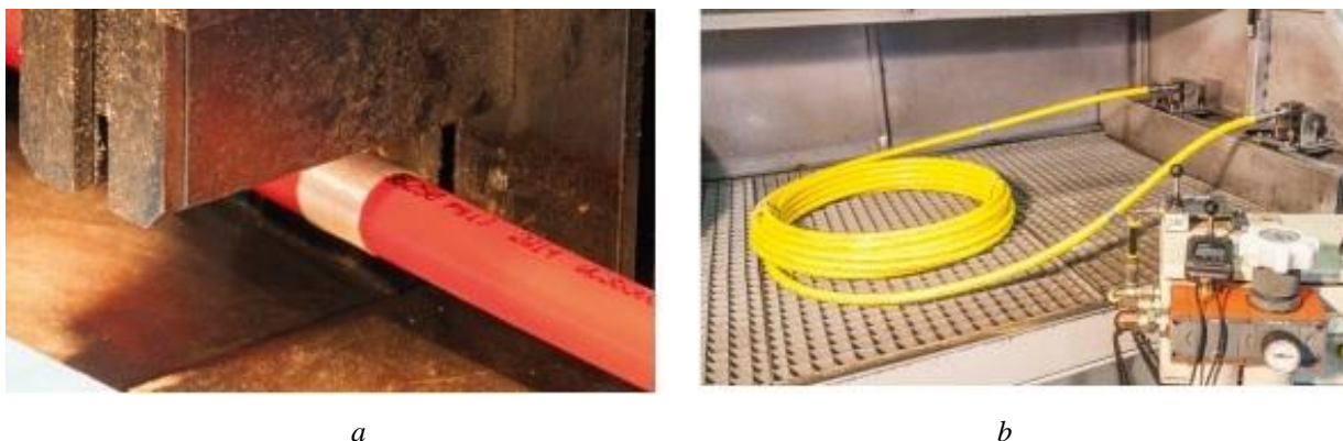
Fig. 4. Technological methods of improving of hoses cutting: a – surface winding by heat-resistant fibrous film; b – supply of compressed air
