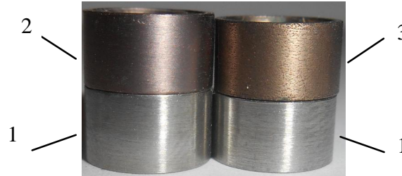
Fig. 8. The general view surface of the Zr-1 %Nb tubes after processing by the modes: 1 – P0, 2 – P4, 3 – P7
