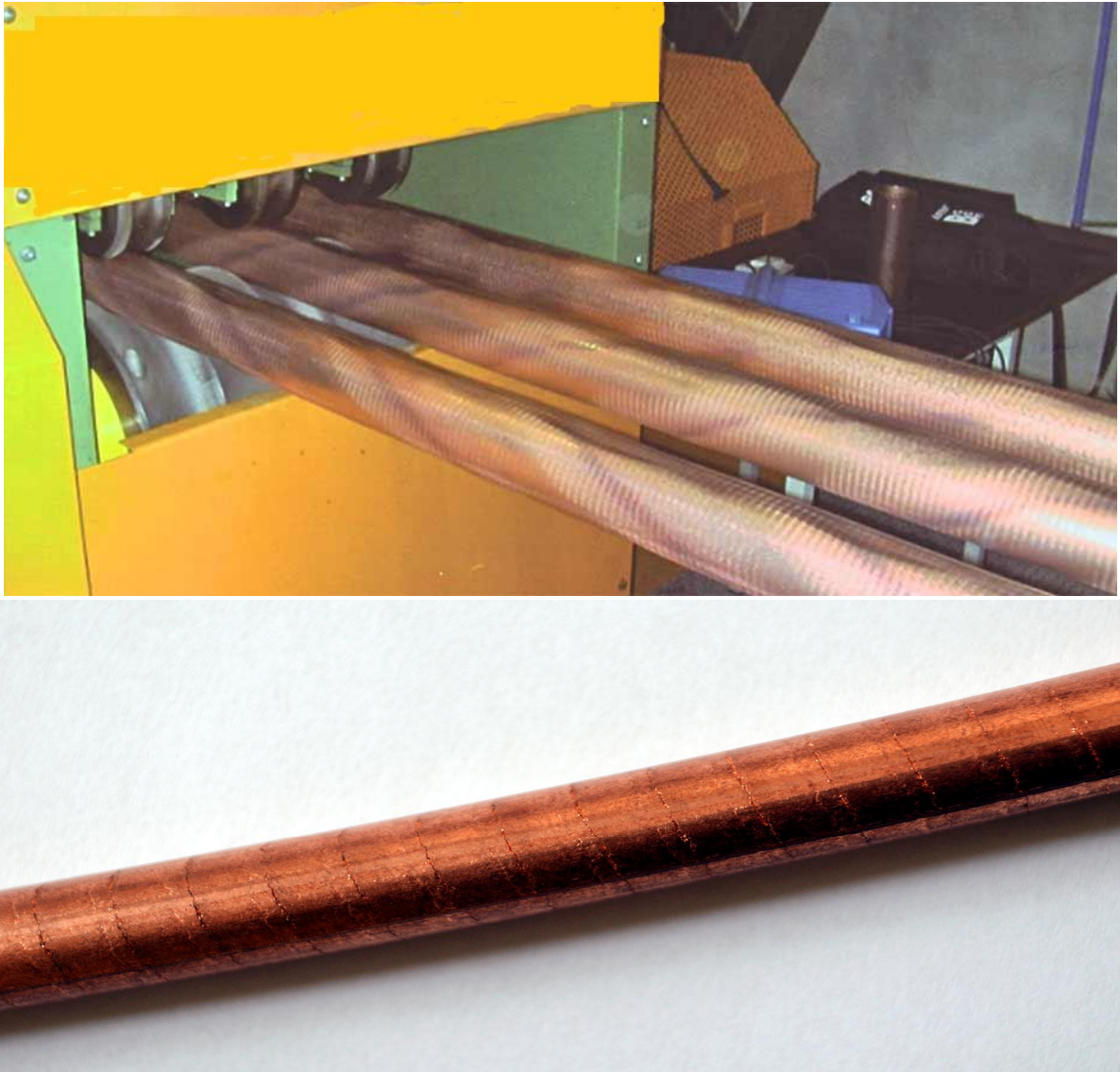
Fig. 1. Horizontal continuous founding [7]
