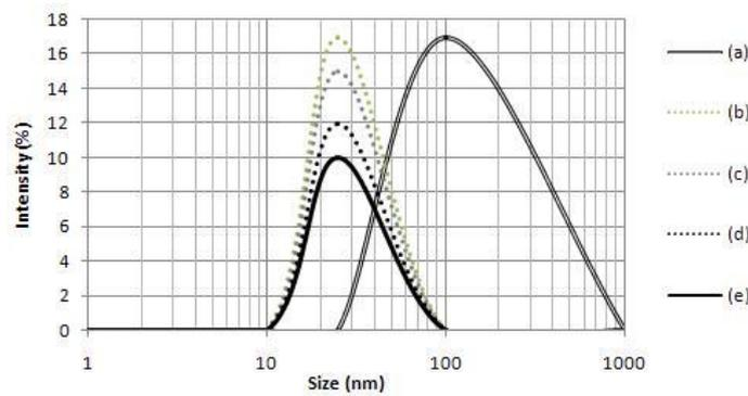
**Fig. 2.** Size distribution of naked Ag NPs (a) and Ag NPs coated with HAS (b), BSA (c), FCS (d), and PNA (e). All nanoparticles were suspended in RPMI-1640 and size distribution was carried out by DLS at 37 °C.
