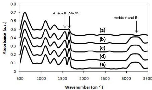
**Fig. 3.** FTIR spectrum of naked Ag NPs (a) and Ag NPs coated with HAS (b), BSA (c), FCS (d), and PNA (e). For FTIR experiment, all nanoparticles were separately dried on KBr and scanned at 500-3500 cm<sup>-1</sup>. Amide band I, amide band II, and amid A&B were seen in all coated Ag NPs.
