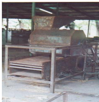
Plate 2 – Locally Developed Rice Thresher
