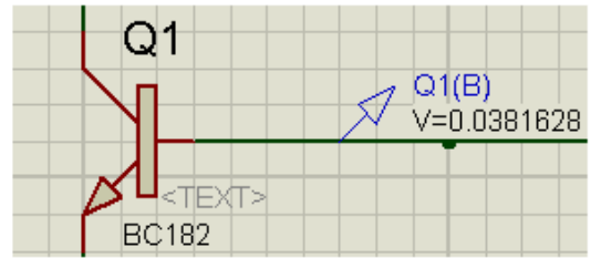
Figure 10b: Q1 turned OFF with base \approx 0
