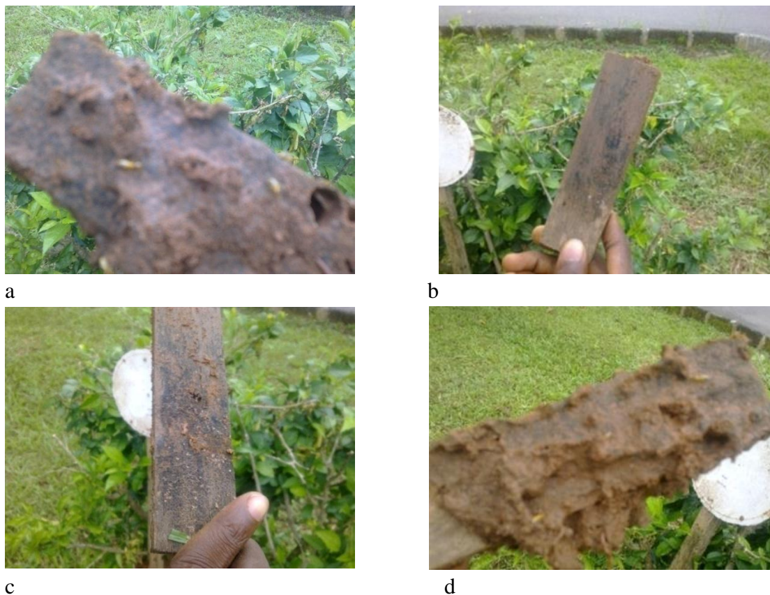
Figure 2: Effect of decay on Ceiba pentadra subjected to Grave yard decay resistance tests after 12 weeks of exposure: (a) untreated wood (control), (b) solignum treated (c) methanol extract treated and (d) water extract treated
