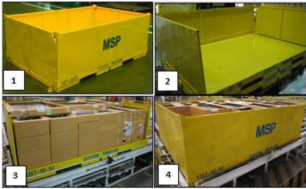
Figure.3 The structurally strengthened returnable packaging (Source: Toyota Motor Thailand)
