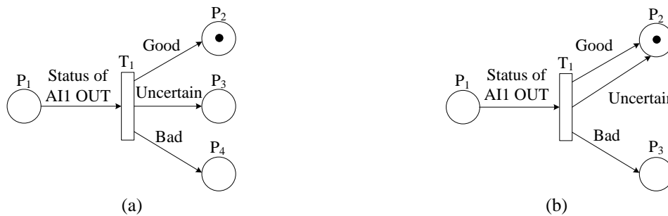
Figure.4 Simple Petri net models for representing behaviors of the FF-based PID control loop: (a) with increased safety and (b) with increased availability
